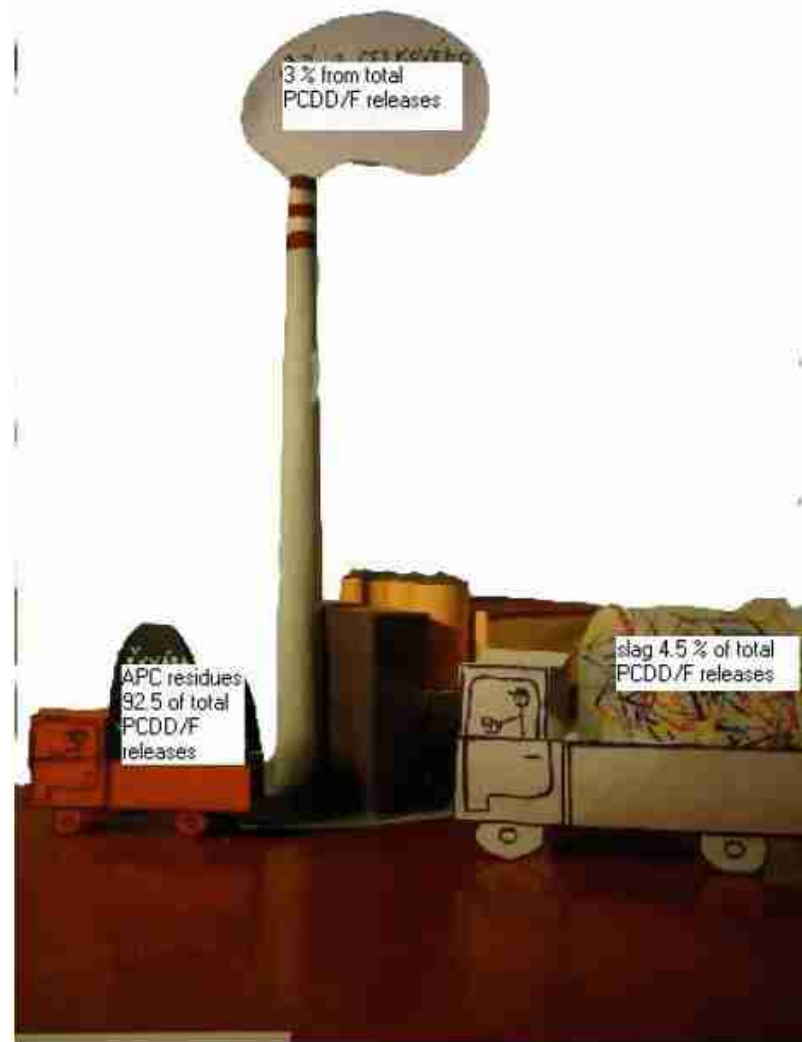
Picture 3: Balance of PCDD/Fs releases into different environment compartments from MWI Liberec.
